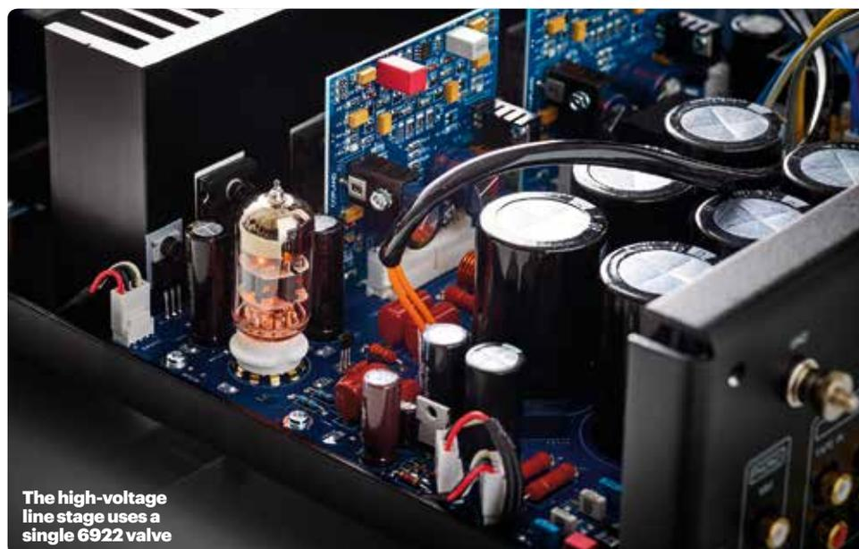
The high-voltage line stage uses a single 6922 valve
