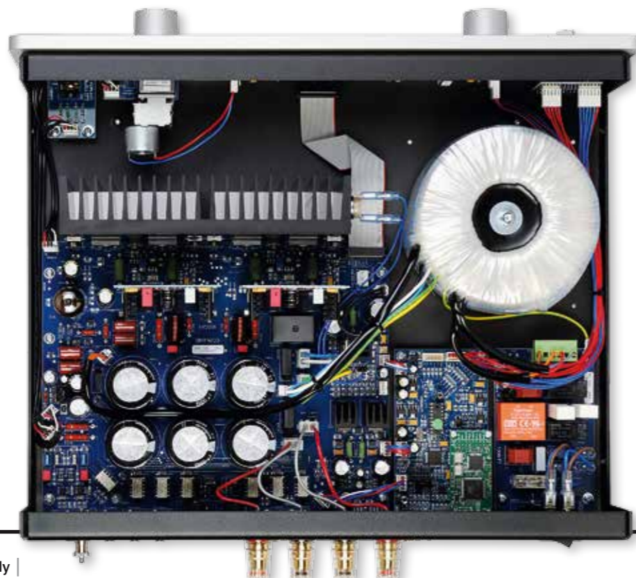
RIGHT: High voltage line stage uses a single 6922 double-triode [left] from Electro-Harmonix while the output stage comprises a pair of high current transistors from On Semiconductors [on heatsink]. Note large toroid [right] and PSU [left]
